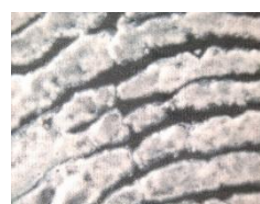
Figure 13; cyanoacrylate makes the use of third level features (pores) not possible.
